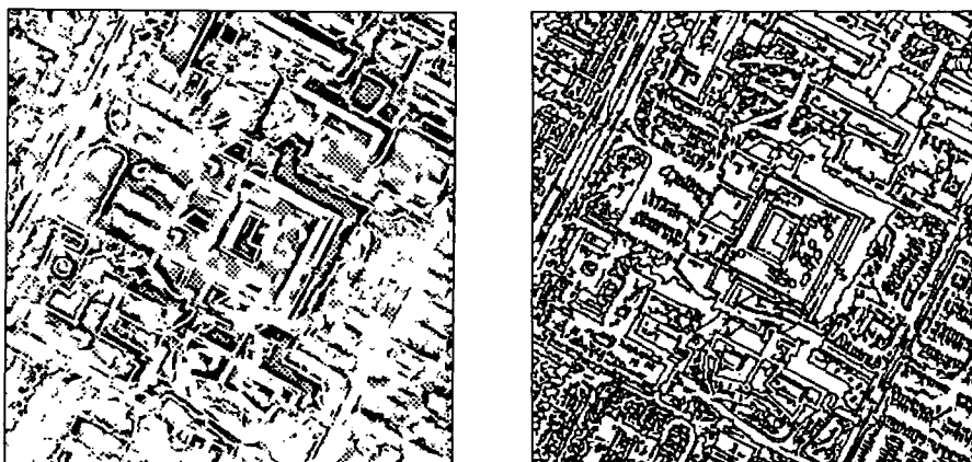
Fig. 10. The edge finder's sign-test map (left; light indicates passing ) and its output boundaries (right), for one of the images in figure 1.
