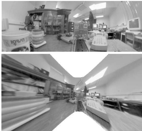
Figure 3: (Top) A 240° degree stereographic view of our lab, creating by rotating the camera into five positions and correcting the resulting images with the new nonparametric distortion algorithm. (Bottom) A 160° perspective image from the same viewpoint, created from three images. Gross expansion of peripheral areas makes perspective unusable for fields of view above 140°.
